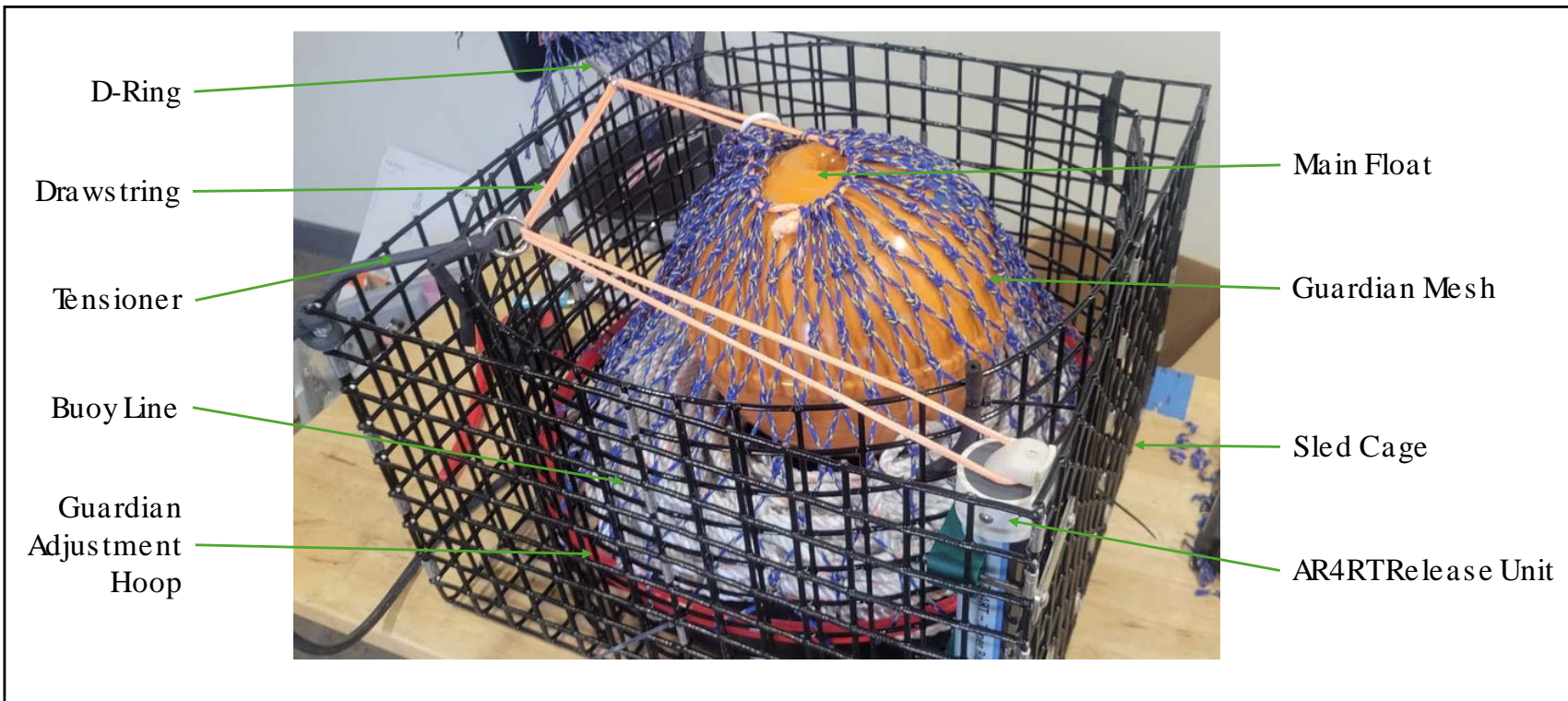
Figure 4. Guardian Sled line handling system.
