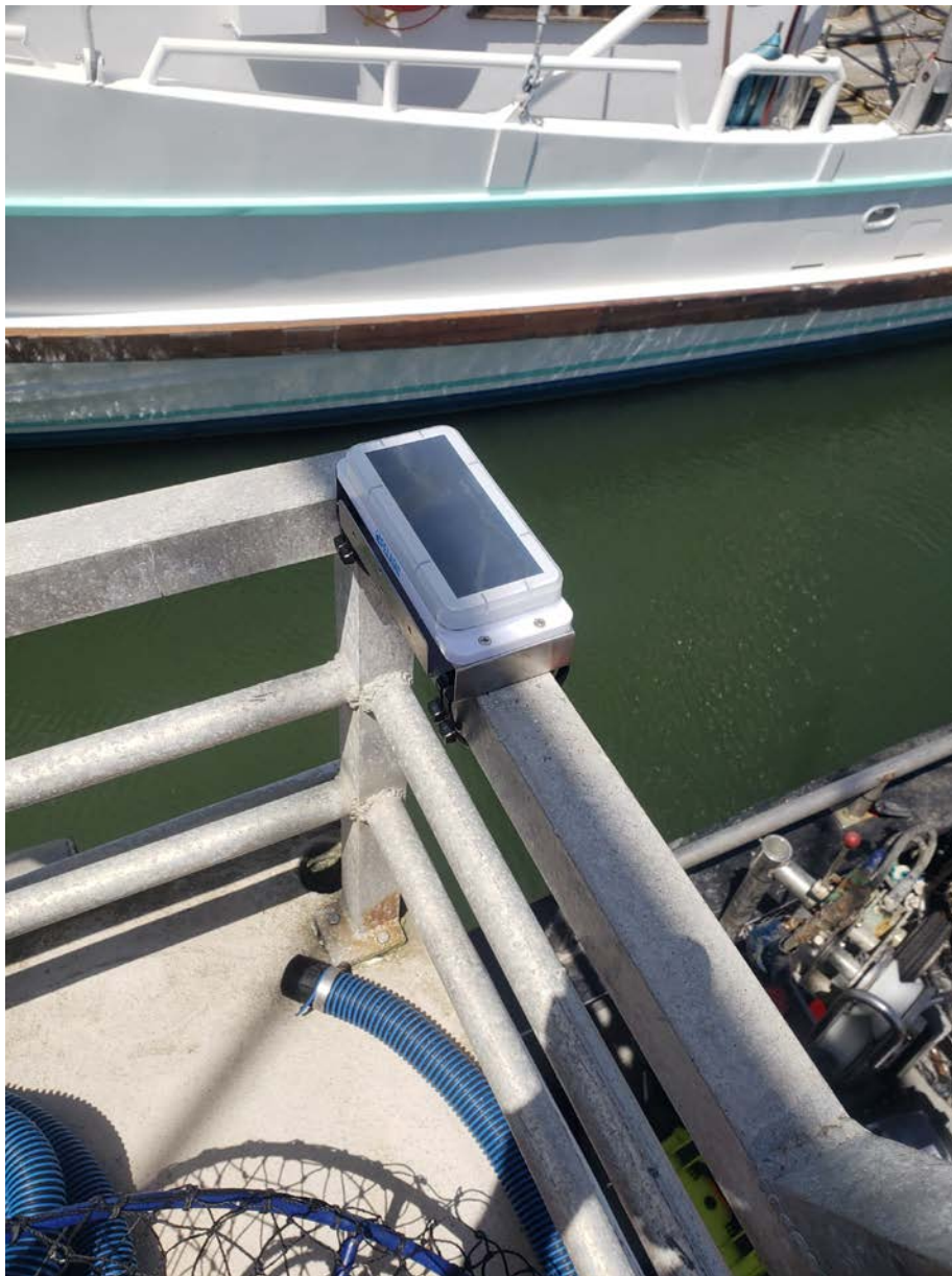
Figure 10. The Pelagic Data Systems Solar Logger installed on a Dungeness crab fishing boat.
