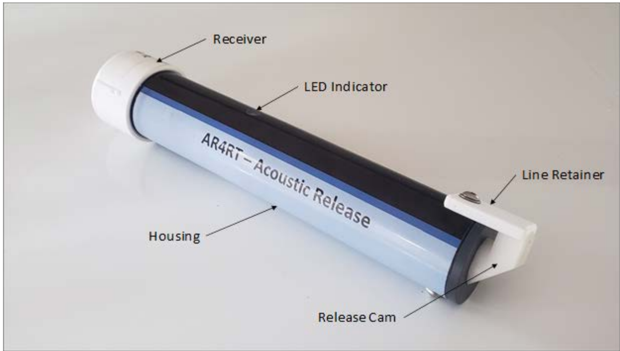
Figure 2. The AR4RT on-demand release unit.
