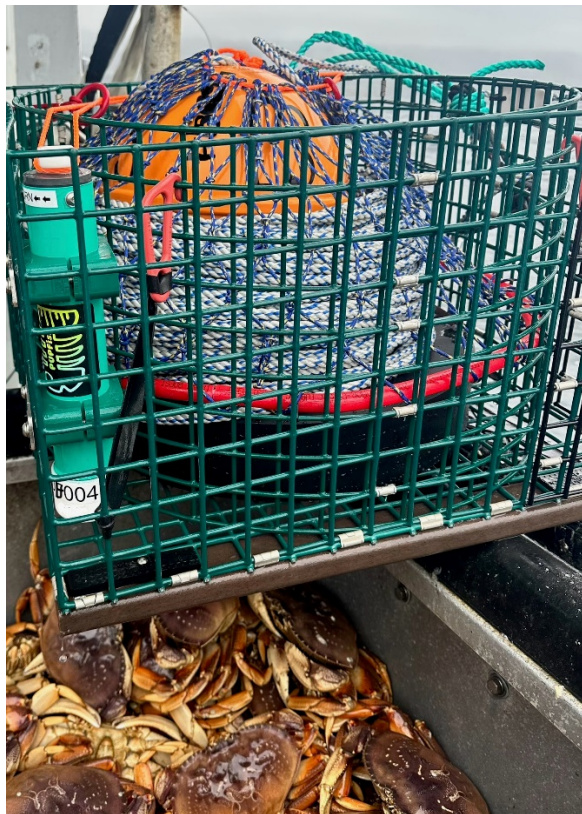
Caption: Sub Sea Sonics acoustic release (left) inside a Guardian Ropeless System sled with line and buoy as tested in the trials, pictured above Dungeness crabs caught with the gear system.
